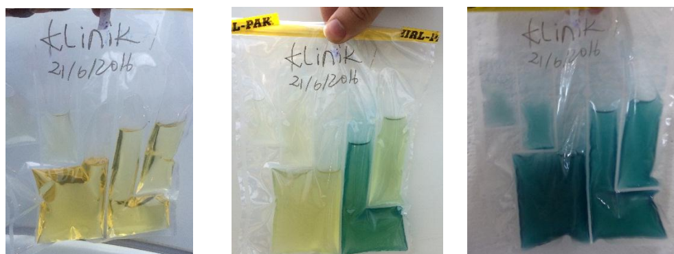
Figure 10 – Example of the water quality test results from the clinic – original test (left), preliminary result shown to community after two days (centre) and fully developed result after four three days (right). Blue colour indicates presence of bacteria
